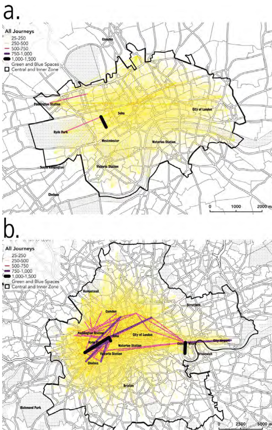
Figure 2. Flows, origin, and destination volumes. (A) Undirected volumes of AddLee trips between TAZs for Central London; (B) undirected volumes of AddLee trips between TAZs for inner and Central London. TAZ = traffic analysis zone. (Color figure available online.)
