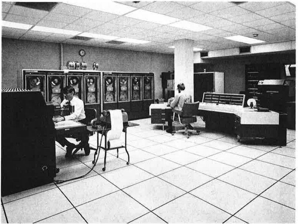
Fig. 16. The computer room of the Coordinated Science Laboratory showing the display unit on the left, tape banks, console, printer, and computer in the far corner.
